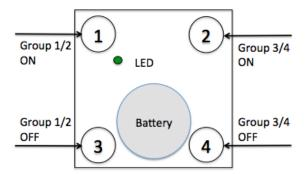
**Control with single buttons** In this mode a group of devices is controlled by a single button: single click turns 'ON'; double click turns 'OFF' devices in the group. In case dimmers are controlled, holding down the button will dim up, click and hold down will dim down the load. The group number corresponds to the button label.
