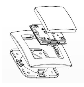
The device can be mounted on every dry and flat surface using either screws or double side adhesive. First the mounting base is fixed on the wall. Next step the switch frame is placed on the 2 frame and the electronic insert is used to fix the frame to the mounting base as shown on the image. Finally the switching paddle(s) are mounted on the electronic base.
