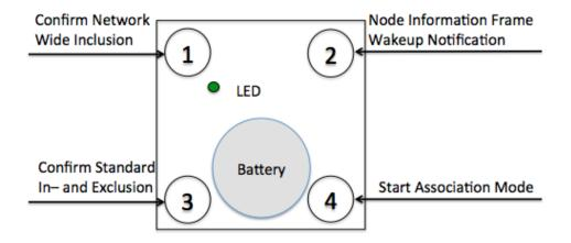
Button 1 - Network Wide Inclusion: The device can be included into a Z-Wave network from any physical location in the network. This requires a primary controller supporting Explorer Frames. This mode lasts for 20 seconds and stops automatically. Any button press stops the mode as well.
